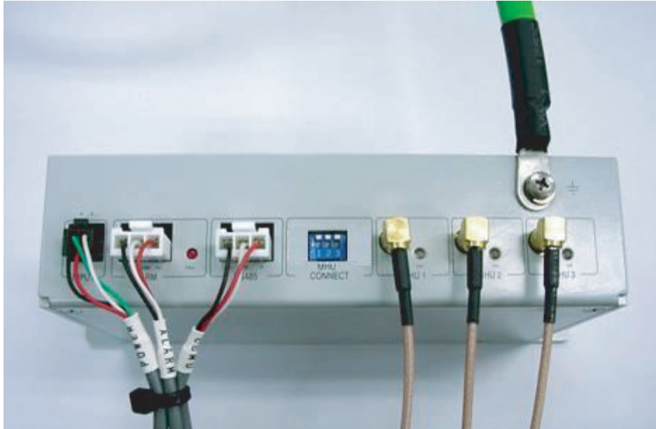
(Left to Right: Power Cable, Alarm Cable, RS-485, Three MHU (Bias-T) Cables, and Ground Cable)
